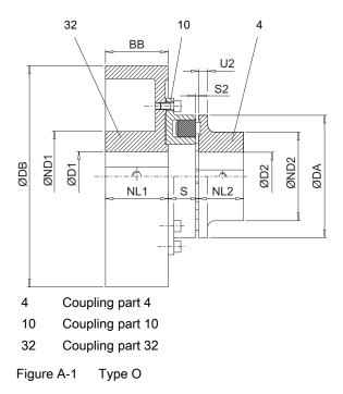
Table A-1 Speeds, geometry data and weights of type O
