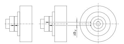
Figure 8-1 Markings for calculating the torsional backlash
